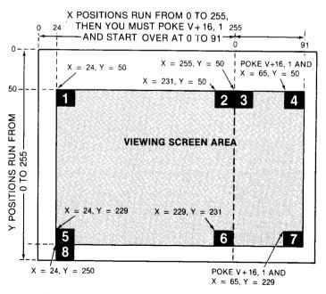
Figure 3-5. Determining X-Y sprite positions.
