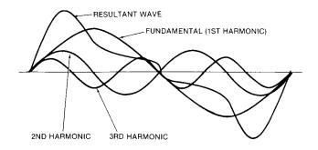
In musical theory let's say that the fundamental frequency is harmonic number 1. The second harmonic has a frequency twice the fundamental frequency, the third harmonic is three times the fundamental frequency, and so on. The amounts of each harmonic present in a note give it its timbre.
