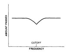
Register 24 determines which type filter you want to use. This is in addition to register 24's function as the overall volume control. Bit 6 controls the high-pass filter (0 = off, 1 = on), bit 5 is the bandpass filter, and bit 4 is the low-pass filter. The low 3 bits of the cutoff frequency are determined by register 21 ( $L_{cf}$ ) ( $L_{cf}$  = 0 through 7). While the 8 bits of the high cutoff frequency are determined by register 22 ( $H_{cf}$ ) ( $H_{cf}$  = 0 through 255).
