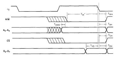
\*TW is measured from the latest occurring of  $\phi_2,\ \overline{\text{CS}},\ \text{R/W}.$
