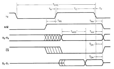
\*T\_{ACC} is measured from the latest occurring of  $\phi_2,\, \widetilde{CS},\, A_0\text{-}A_4.$
