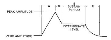
This volume envelope can be easily reproduced by the ADSR as shown below, with typical envelope rates:
