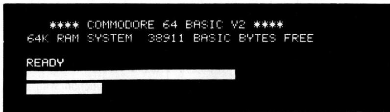
Now, hold **CTRL** while depressing any of the other number keys. Each of them has a color marked on the front. Anything displayed from this point will be in that color. For example, hold **CTRL** and the **8** key and release both. Now hold the **SPACE BAR**.
