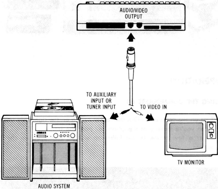
If you purchased peripheral equipment, such as a VIC 1541 disk drive or a VIC 1515 printer, you may wish to connect it at this time. Refer to the user's manuals supplied with any additional equipment for the proper procedure for connecting it to the computer.
