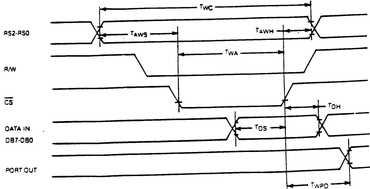
Note: All timings referenced to  $V_{IL\max}$ ,  $V_{IH\min}$  on inputs and  $V_{OL\max}$ ,  $V_{OH\min}$  on outputs.
