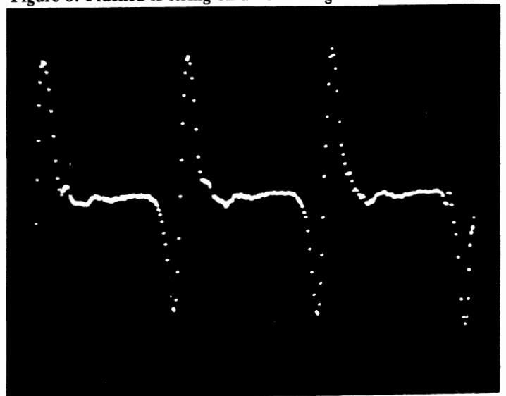
Figure 8. Plucked A string on an electric guitar.
