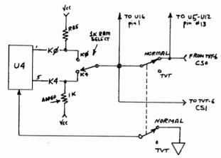
The SPDT switch selects whether the KIM 1K RAM is at 0000 hex to 03FF hex (with the 4K RAM removed!) or at 1000 hex to 13FF hex (with the 4K RAM present)
