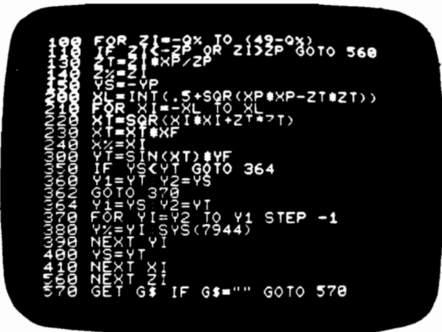
Figure 3: The problem has been corrected by drawing a line between plot points and eliminating the gaps.
