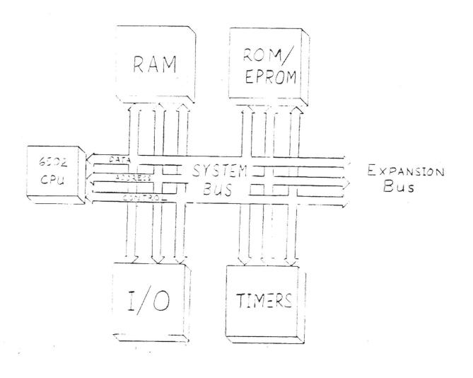
Figure 1-1. Model 6500 CPU Board Block Diagram
