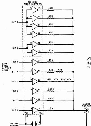
Fig. 4. Simple 8-bit digital-to-analog converter.
