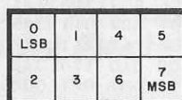
Fig. 7. In high-resolution mode, each memory byte is used to represent 8 picture elements.
