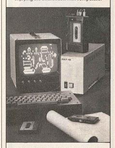
The POLY 88 System uses a video monitor for display, a keyboard for input and cassette tape for storage. The system will also connect to a hard-copy terminal. Poly 88 hardware consists of an 8080 based CPU circuit card with onboard memory and I/O, video display circuit card with keyboard input port and graphics capability, and mini-cards that connect to the CPU board via ribbon cable for cassette or serial
