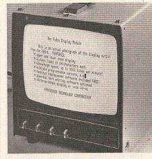
character to the end of the screen; program control for scrolling in increments of one to 16 lines without rewriting memory; and "windowshade" blanking of the text above the desired starting location under program control.
