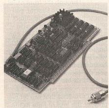
HE TYPE of computer busline used in the Altair 8800 and Imsai 8080 has become one of the most popular elements in the area of hobby type minicomputers. A number of devices have been designed to plug directly into this bus, a very useful one being the Processor Technology Model VDM-1 video display module, which occupies a single slot in the computer.
