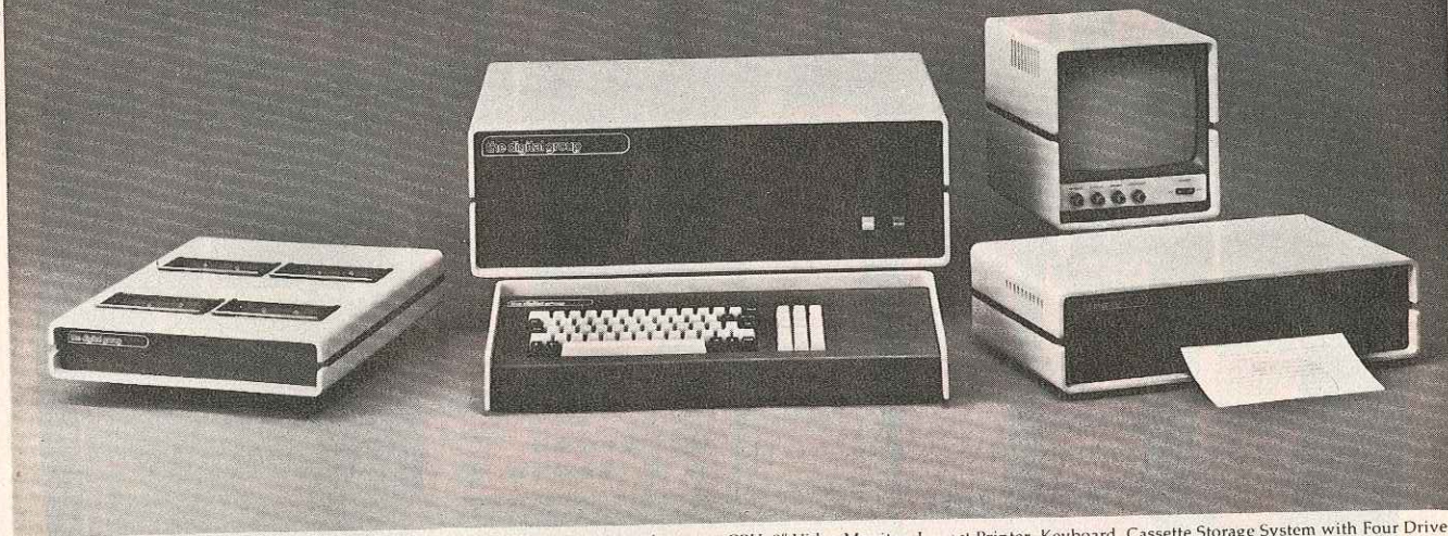
Clockwise from top: CPU, 9" Video Monitor, Impact Printer, Keyboard, Cassette Storage System with Four Drives.
