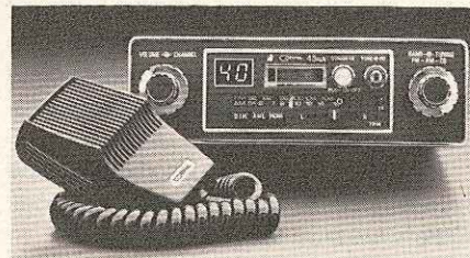
Cobra 45XLR combines 40-channel CB with AM/FM/stereo FM.
