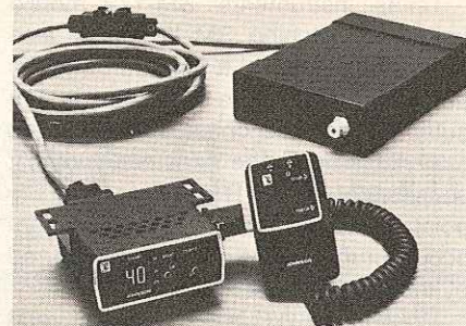
Johnson 4330 has remote control mike with speaker and channel indicator in separate box.
