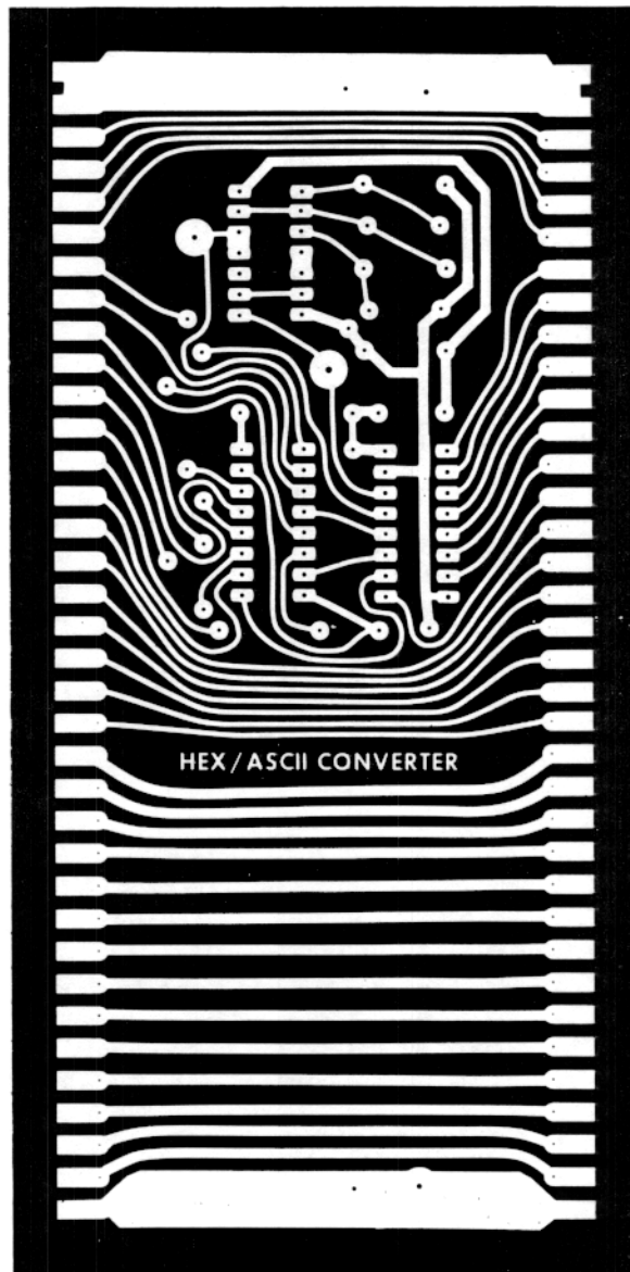
Fig. 4. Actual-size etching and drilling guide (right) and component layout (above) for the pc board. The board is connected between the TVT-6 and the KIM-1 microcomputer.
