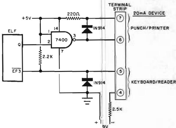
Fig. 2. Interface between Elf and a 20-mA current-loop device such as a TTY.
