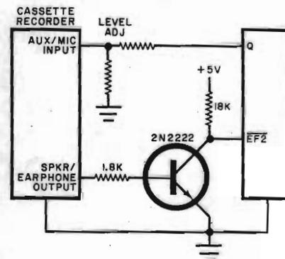
*Fig. 1. Simple interface between Elf and cassette recorder.*
