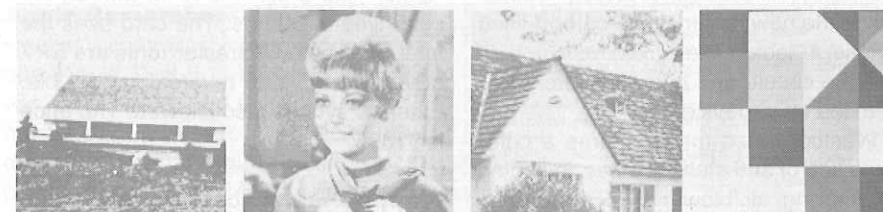
This is the kind of resolution obtained from Vector Graphics video board.
