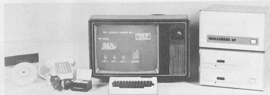
Ohio Scientific C8P DF System—Challenger 8P Computer, dual-disk drive, terminal, monitor, peripheral control devices.
