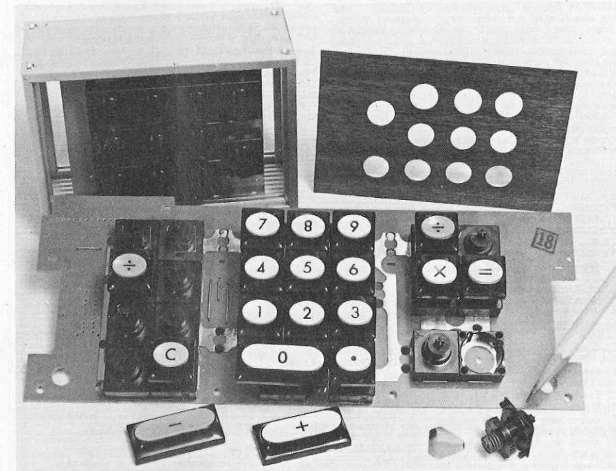
Desktop calculator keyboard can be cut apart to make smaller keypads. The pencil at right points to removed top part of keyswitch. Topside brass stampings form part of switch and key strings.
