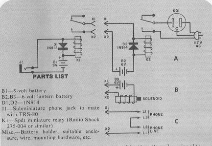
Fig. 1. When computer gets correct combination, it sends a signal to energize K1, which can control other circuits as in A, B, and C.
