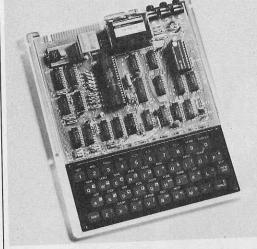
Photo of the ZX80 with its cover removed shows the compact assembly that was used to achieve its small size.
