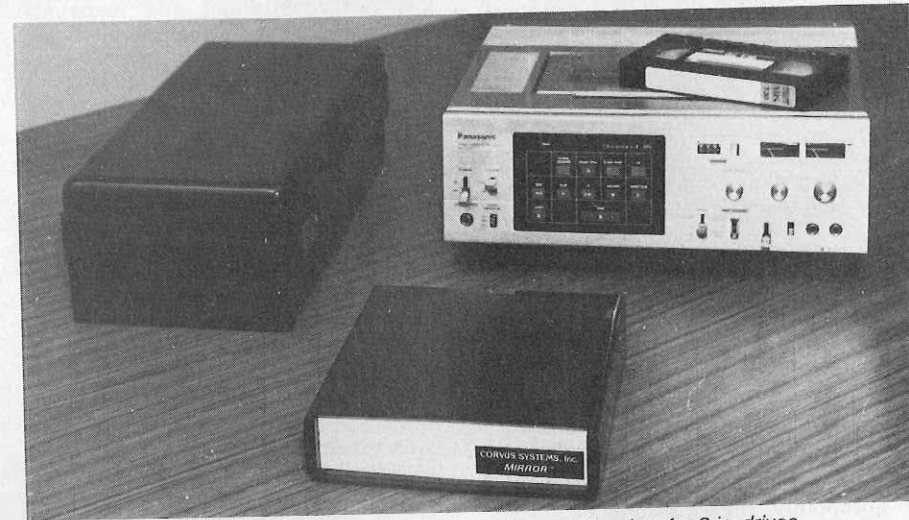
Corvus Mirror and VHS tape system provide tape backup for 8-in. drives.
