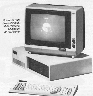
ing Greek, foreign language special characters, and mathematical symbols. The graphics display format is 640 dots wide by 250 (or 200) dots high, fully addressable array; or 320 dots wide by 250 (or 200) dots high, with 4-level grey scale. The I/O includes the RS-232C standard with an asynchronous 75-to-19.2K baud rate or synchronous 100K with bisync and bit-oriented protocols. The parallel port is compatible with IBM/Epson or Centronics printers.
