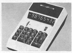
The overall range of the calculator is from 0.0000001 to 99999999. If the instrument's capability is exceeded-either during entry or during totalling-the keyboard automatically locks out, and the extreme left readout displays an E.
