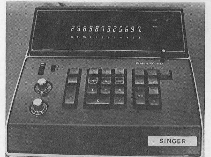
A LATE MODEL DESK CALCULATOR, the Friden EC 1117 has memory capability. Low-cost machines like this are popular with businesses. Friden also manufactures printing calculators and all electronic cash registers.
