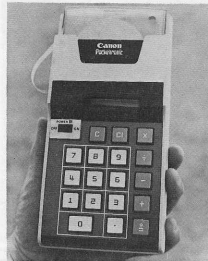
THE CANON POKETRONIX is the only portable electronic calculator with a paper tape printout. This novel machine incorporates Texas Instruments MOS LSI circuitry but is manufactured in Japan. Texas Instruments also manufactures the semiconductor thermal printout device. The paper tape can be replaced almost instantly by plugging in a new cassette.
