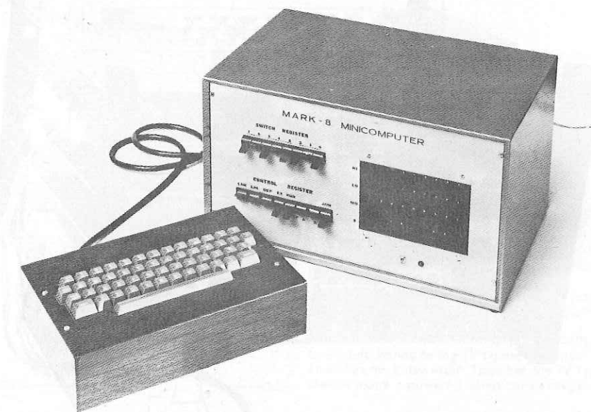
COMPUTER WITH ASCII KEYBOARD makes a complete working computer system. You can use the computer without the keyboard, but it is more difficult.
