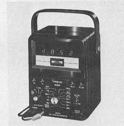
FIG. 19—SON OF 260 is the Simpson model 360 digital vom.
