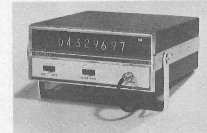
FIG. 6—THIS FREQUENCY COUNTER has eight digits in its readout and goes out to 120 MHz.
