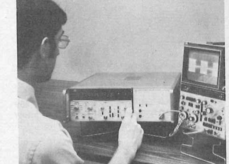
FIG. 8—HIGH-FREQUENCY MEASUREMENTS can be made with instruments like H-P 5354A. It goes to 4 GHz.
