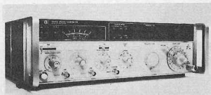
FIG. 10—VHF SIGNAL GENERATOR (450 kHz to 550 MHz) has digital readout to show what frequency signal it is producing.
