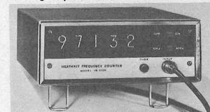
FIG. 5—HEATHKIT MODEL IB-1100 frequency counter uses Nixie type readout.
