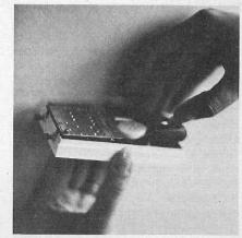
BATTERY CHANGE PROCEDURE, Grasp the unit about one-third the way down. Pull halves apart, keeping them as parallel as possible when separating. Lift battery up and out at connector end, as shown above.
