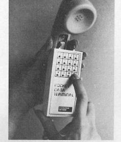
USING THE POCKET DATA TERMINAL with a telephone. Be sure the nickel-plated grommet on the rear of the unit is centered over and touches the microphone of the phone (or two-way radio). The gain of the system receiving the signal determines whether the volume boost (right top button) should be used.
