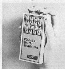
PRESSING THE LEFT BUTTON on the Pocket Data Terminal starts it into Auto-Dial operation-pressing the right button boosts the output volume level. Hold both buttons down until the sequence is complete
