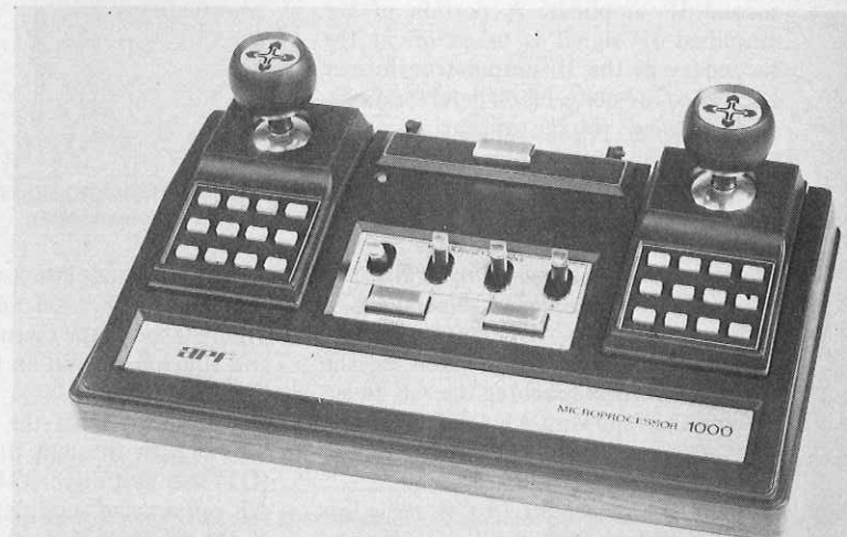
APF'S M-1000 MICROPROCESSOR shown at the right includes both keyboard and joystick controls. Cartridges for both games and educational purposes are available.
