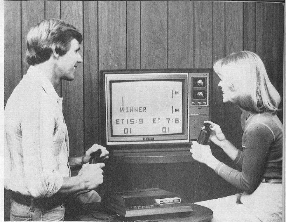
FAIRCHILD'S VIDEO ENTERTAINMENT SYSTEM was the first programmable unit to appear. It uses Videocart cartridges to set up the games. Current games include Tic-Tac-Toe , Desert Fox , Spitfire , Black Jack , Baseball and Space War . Others are on the way.
