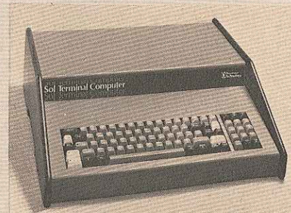
SOL TERMINAL COMPUTER has computer and alphanumeric keyboard in a single enclosure.
