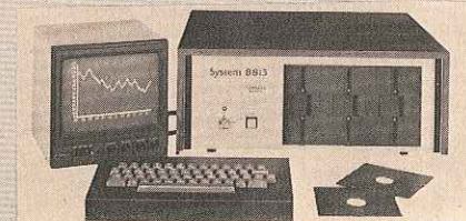
SYSTEM 8813 from Polymorphic has three floppy disk drives.
