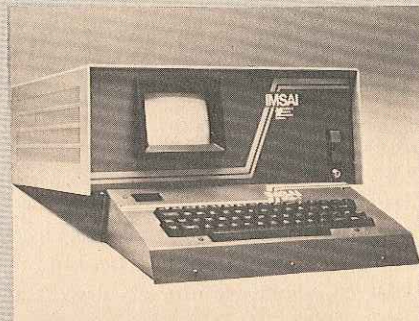
IBK-1 MICROCOMPUTER from IMSAI has built-in card cage, CRT terminal and power supply
