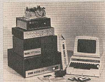
SOUTHWEST TECHNICAL'S 6800 system has optional floppy disc, printer and CRT terminal.
