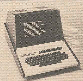
H9 CRT TERMINAL from Heathkit has CRT display plus alphanumeric keyboard.
